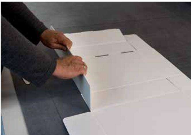
2. Now the cardboard is bent over completely (180°) toward the middle of the cutout along the creased lines. The material has a natural inner restoring force which is thus disabled or at least reduced such that assembly of the finished box is made possible and a perfectly rectangularly-shaped box can be formed. Especially those boxes with long sides tend to bow where this restoring force is not sufficiently broken at these points.
